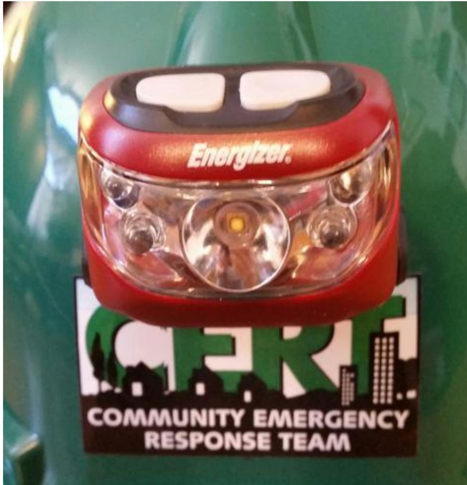
This headlamp has modes for both bright and dim on the main white lamp in the center, two outer white lamps, and two outer red lamps. The red lamps are important if you are in the dark and are trying to read some documentation, or write something, but you don't want the bright white splash-back interfering with your eyes when they are adjusted for darkness. It's also a courtesy when directly facing others:
