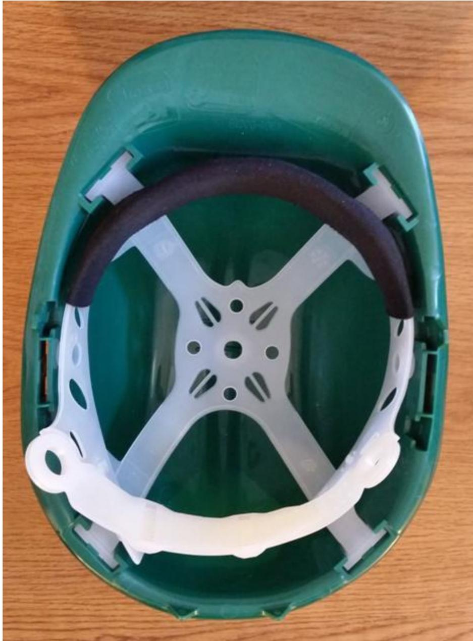
By adding a piece of Velcro loop material to this plastic piece, I now have a much more comfortable area of the helmet resting on the top of my head:
